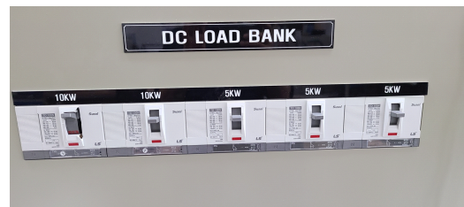
Fig. 10. DC load bank for the scale-down real test.
